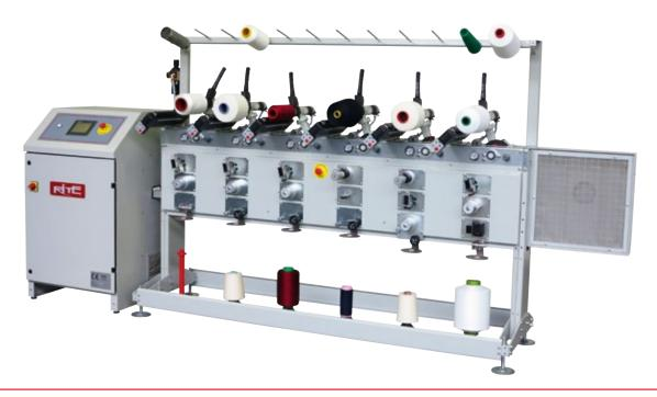
You can also install the "Individual Counterweight System" where it is possible for each spindle to adjust the requested counterweight pressure, by individual manometers, instead of a single one that controls the entire winding units. This system allows more flexibility on the machine! It is also suitable for fitting socks on the package.
